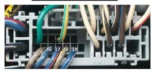
This is the view of the radio connector in the vehicle (note: wire colors may vary between vehicles)
