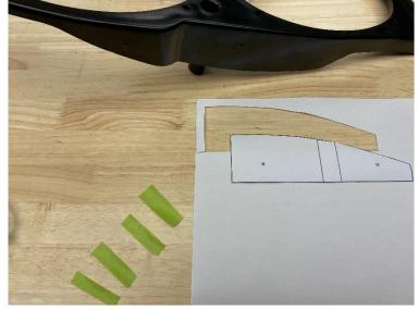
3. Lineup Template to outside edge of speaker assembly. Follow taper until the two lines, meet the contour of the speaker assembly. Starting at the front, tape down as seen in photo.
