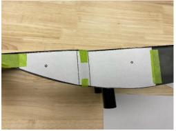
4. Using a 3/32" drill bit, drill out the centers of 2 holes of the template.
