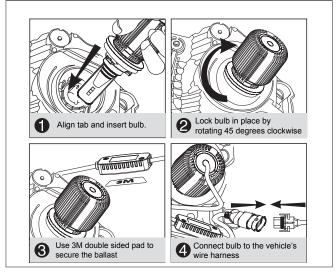
After installation of LED bulbs, adjustment of the headlamp assembly may be required to achieve proper beam pattern. Adjust headlamp assembly in accordance with vehicle's operating manual.
