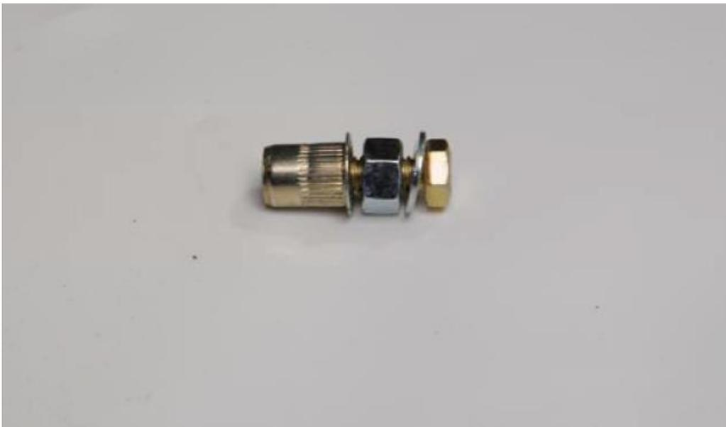
8. Add a silicone bead around the ribs of the riv-nut and place the riv-nut assembly into the drilled hole in the door jam.
