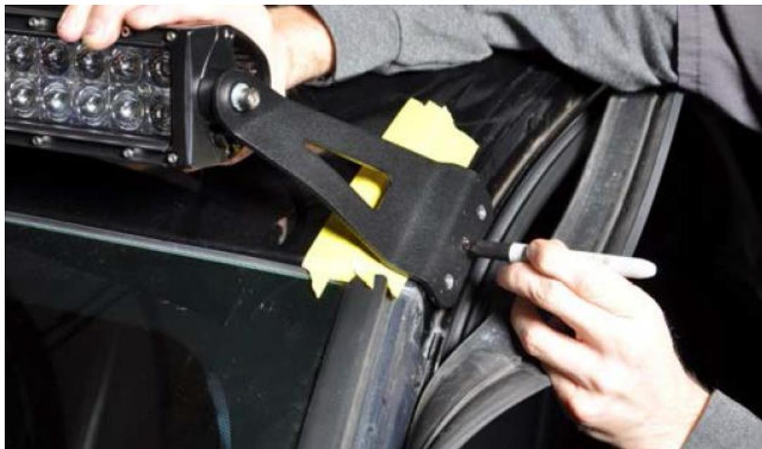
5. Remove the mounts from the truck and drill the previously marked holes with a  $\frac{1}{4}$ " drill bit making a pilot hole.
