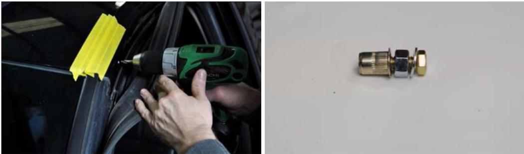
8. Place that assembly into the drilled hole in the door jam.
