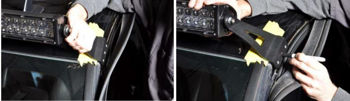
5. Remove the mounts from the truck and drill the previously marked holes with a  $\frac{1}{4}$ " drill bit making a pilot hole.
