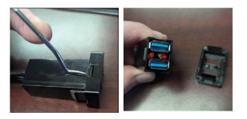
**Step 2:** Using a pick or pry tool remove the back cover of the USB housing.
