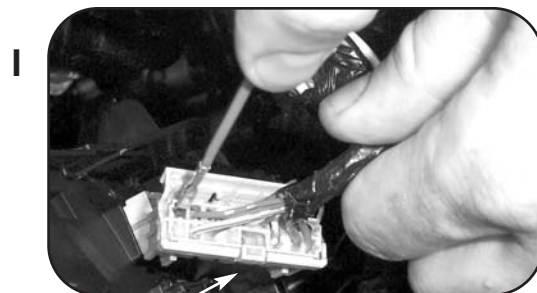
Locking clip on 16-way plug
