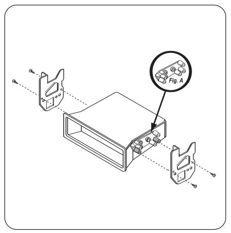
Mount the factory brackets to the *shaded bosses* (Fig A) with **(4) #8 x 1/4" Phillip** screws supplied and mount the entire assembly to the sub-dash.
