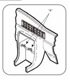
2 Re-connect the battery terminal and test the unit for proper operation. Slide the head unit/kit assembly into the sub-dash until the *Carriage Bolts* engage the mounting slots in the sub-dash shelf and the side tabs on the *Radio Housing* rest against the walls of the sub-dash cavity. (Be sure the rear support bullet on the *Mounting Bracket* engages the rear support hole in the sub-dash). Tighten the *Keps Nuts* onto the bottom of the sub-dash shelf.
