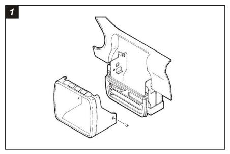
Disconnect the negative battery terminal to prevent an accidental short circuit. Remove (2) pop-clips from the sides of the radio trim bezel. Unclip the radio trim bezel, disconnect the switch wiring and remove the bezel. Remove (2) 7mm hex-head screws securing the top of the factory head unit and disconnect the wiring.
