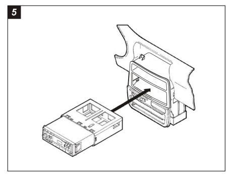
Slide the DIN cage into the kit and secure by bending the metal locking tabs down. Slide the aftermarket head unit into the cage until secure. Re-connect the battery terminal and test the unit for proper operation.
