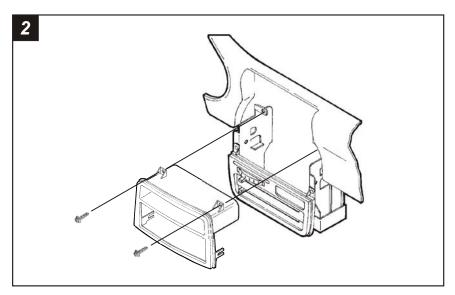
Mount the *Radio Housing* to the sub-dash with (2) 7mm hex-head screws previously removed in step #1.
