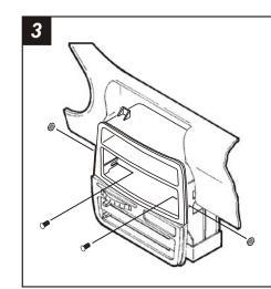
Reach through the *Radio Housing* and mount the lower Housing tabs to the sub-dash with (2) *Captive Studs* and (2) *Pal Nuts* supplied.
