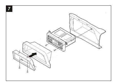
Re-connect the battery terminal and test the unit for proper operation. Mount the head unit/kit assembly to the sub-dash with (2) screws. Place the *Faceplate* into the dash trim bezel and mount with (3) 3/8" *Phillips screws* supplied.
