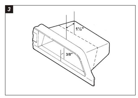
Using the dimensions above, cut and remove the rear portion of the factory pocket from the radio trim bezel.
