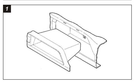
Disconnect the negative battery terminal to prevent an accidental short circuit. Open the glove box and remove (2) Phillips screws securing the right edge of the dash trim bezel. Remove (5) screws from the bottom of the dash trim bezel. Pull out on the upper edge of the bezel and remove.
