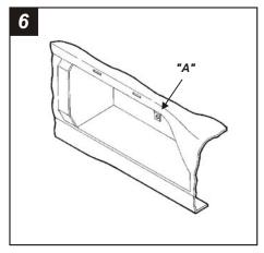
Locate the upper dash tab in the sub-dash and bend the tab down. ("A")
