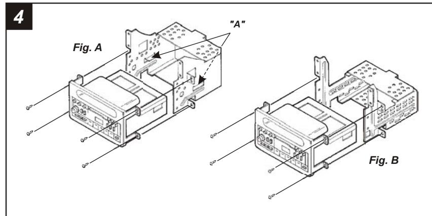
**VILLAGER 1993-95, QUEST 1993-95:** Bend down tabs "A" on the factory radio housing until they are flush with the walls of the housing. Re-connect the battery terminal and test the unit for proper operation. Mount the head unit/kit assembly to the sub-dash (through the holes in the factory radio housing) with (4) Phillips screws previously removed in step #1. (see Fig. A)
