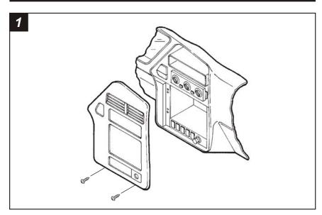
Disconnect the negative battery terminal to prevent an accidental short circuit. Remove (2) screws from the base of the radio trim bezel. Unclip the bottom edge of the radio trim bezel and disconnect the hazard light, defroster, wiper and cligarette lighter wiring. Remove the radio trim bezel. Remove (4) screws securing the factory head unit and disconnect the wiring.
