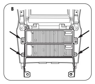
4 Attach the assembled units and brackets to the radio trim panel using the factory screws removed during disassembly.
