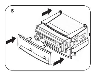
4 Attach the radio / housing assembly to the radio trim panel using the factory screws removed during disassembly. (Figure C)
