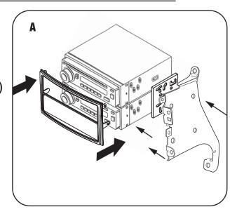
Removed from radio during disassembly) on the left side of the ISO units. Align the pins on the trim-plate with the holes on the factory bracket and mount the factory bracket to the ISO units using screws supplied with the radio. (Figure A)
