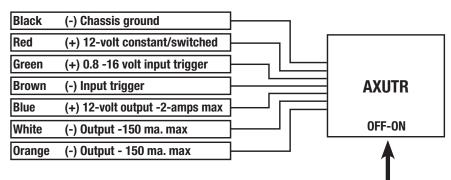
Programming switch must be turned off after the AXUTR is programmed!
