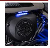
Use Y cables and extensions (not included) to connect strips to existing kit. Route cables, avoiding moving parts, hot surfaces, and pinch points. Make sure to secure cable and any excess.
