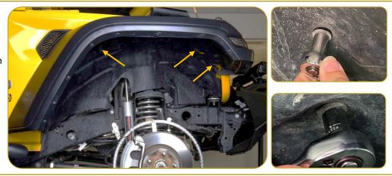
2. Using a panel removal tool, pull out the 5 Christmas tree clips. Pull the inner fender liner back, starting at the front to expose light housing and wiring.
