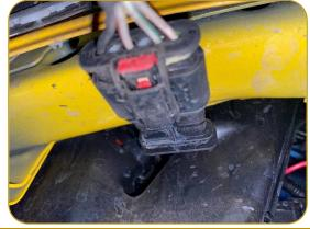
7. Clip new harness into fender, and reinstall light assembly into fender in reverse order of removal.
