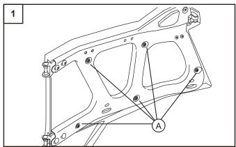
1. Remove five original factory screws A from vehicle door frame. Save the screws A.
