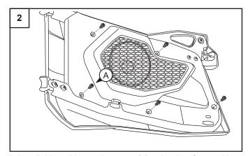
2. Install driver side speaker cover [1] to the door frame with five screws A.
