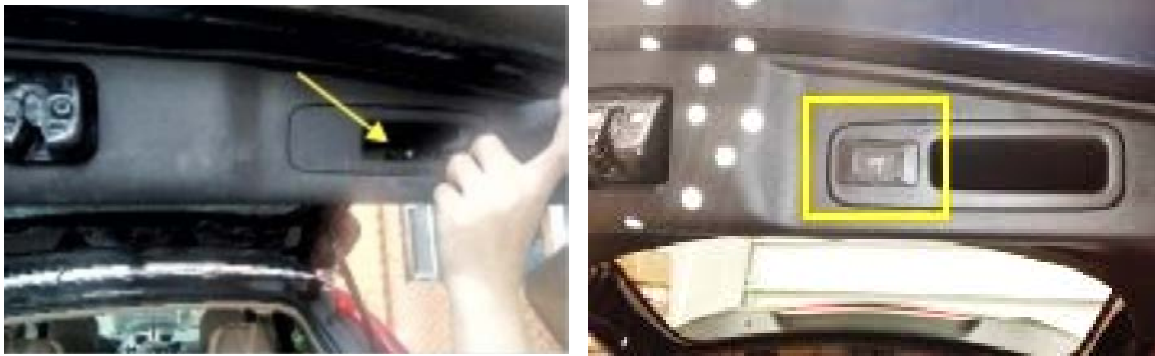
16. Remove the screw in the handle pocket. Remove the handle pocket. Use the provided hole saw to make a hole in the blank space on the pocket front for the rear button.
