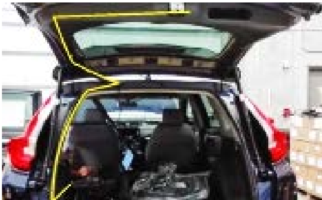
17. Run the wiring for the button as shown in the photo.
