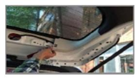
2. Remove the side panels on both sides of the tailgate.
