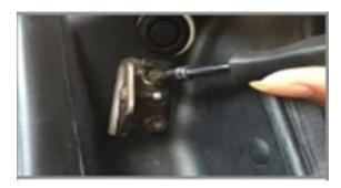
7. Replace factory brackets with the new brackets using the OE screws.
