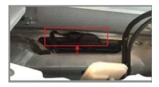
10. Unplug the connector from the factory handle and place the t-harness inline.
