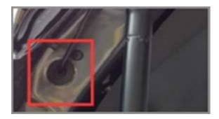
9. Use this grommet to run the wiring for the powered struts.
