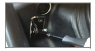
6. Remove the factory bracket by removing the two screws.
