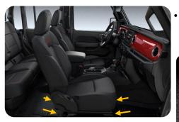
Locate the (4) T50 Torx bolts holding seat into place and remove
